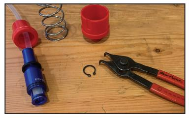
2. Separate the adaptor from the probe. The spring, outer collar, slip ring, and seal ring may now be removed from the assembly. Clean all parts using contact or brake cleaner and compressed air. Carefully inspect all components for wear or damage, and replace if necessary.
