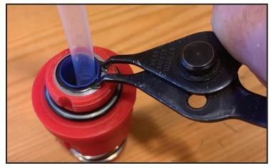
1. Carefully remove the circlip using external circlip pliers, simultaneous holding the adaptor securely to prevent the spring from ejecting the adaptor from the probe.
